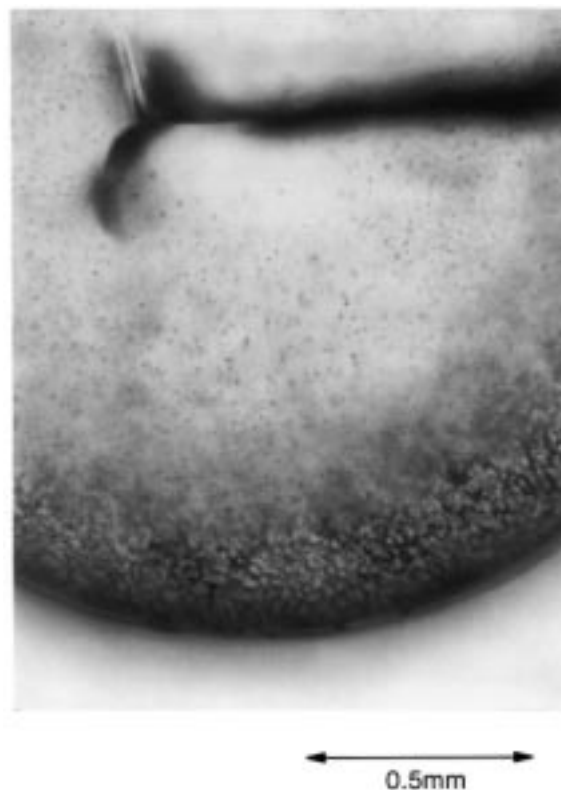
Fig. 2. Microvoids (black points) observed at the growth length of 18 mm in a 22 mm long undoped YAG fiber grown in \text{Ar} + 2\%\text{O}_2 . A significant accumulation of microvoids is seen at the periphery of the fiber. Cracks exist in the upper part of the photograph.
