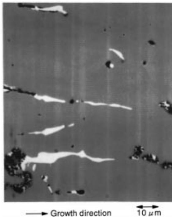
Fig. 3. SEM micrograph (back-scattered electron image) of Y 2 Ti 2 O 7 precipitates (white phase) in the Ti-doped YAG fiber (TY-3A) grown from a 2.5at.% Ti-doped feed rod in pure Ar atmosphere.
